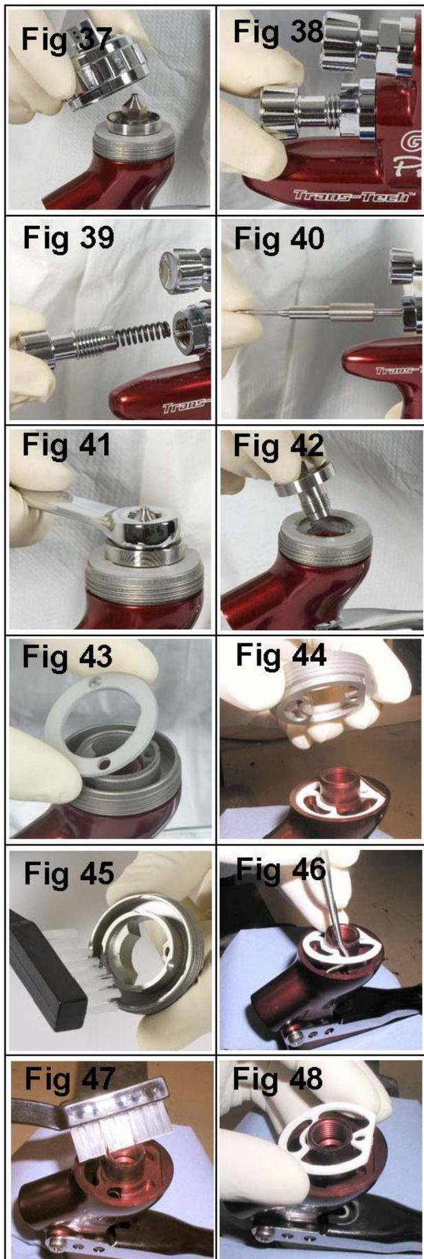
1. Remove air cap and retaining ring. (See fig 37)
