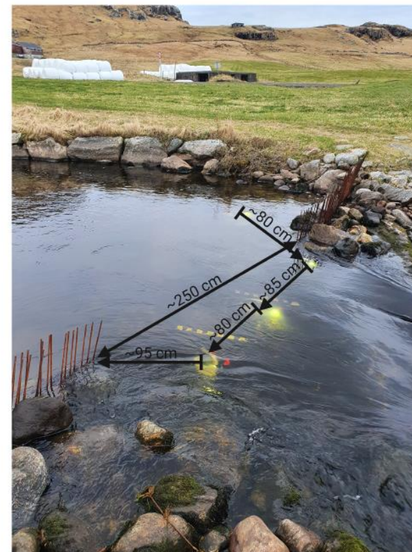
FIGURE 2 Camera array with measured distance between camera platforms. All cameras had overlapping line of sight for maximum detection probability of passing fish. Created in https://BioRender.com .
