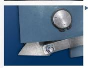
► SAFETY Device allows wires to rest without load, increasing the safety and minimizing wear
