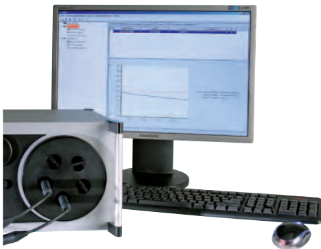
HydroGen2 chamber door with up to 5 probe ports. External monitor with HW4 software.
