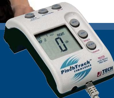
From standard to custom pinch tests, PinchTrack Commander is the industry standard for collecting pinch strength data.
