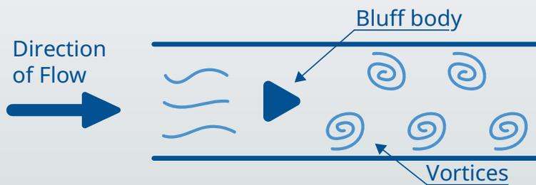
Figure 1: Vortex Flow Measurement
