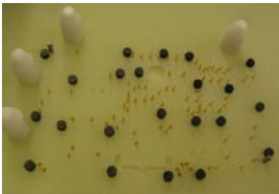
Customized Probe Plate Unit (KTE) with Spring Loaded PCB Support Plate (PRA)
