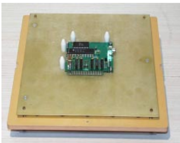
Replacement Kit to PAZ 200 with spring-loaded PCB support plate
